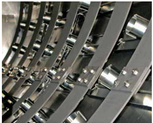
Fig. 2. Lightweight, curved graphite elements are the most popular choice for general heat-treating and brazing applications
