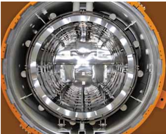
Fig. 1. Modular hot zone within vacuum chamber showing heating elements, insulation, supporting structure and hearth
