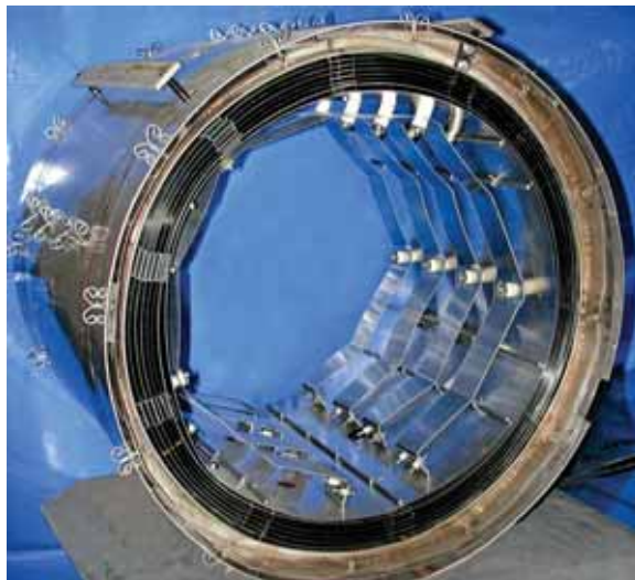
Fig. 4. Hot-zone support structure
