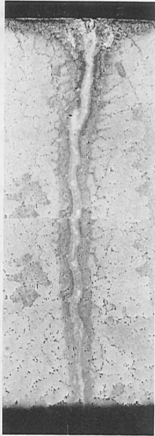
Figure 9. FCP cleaned and brazed filled crack - etched. Shows clean, oxide free and well filled repair C-1023. (MAG x 50)
