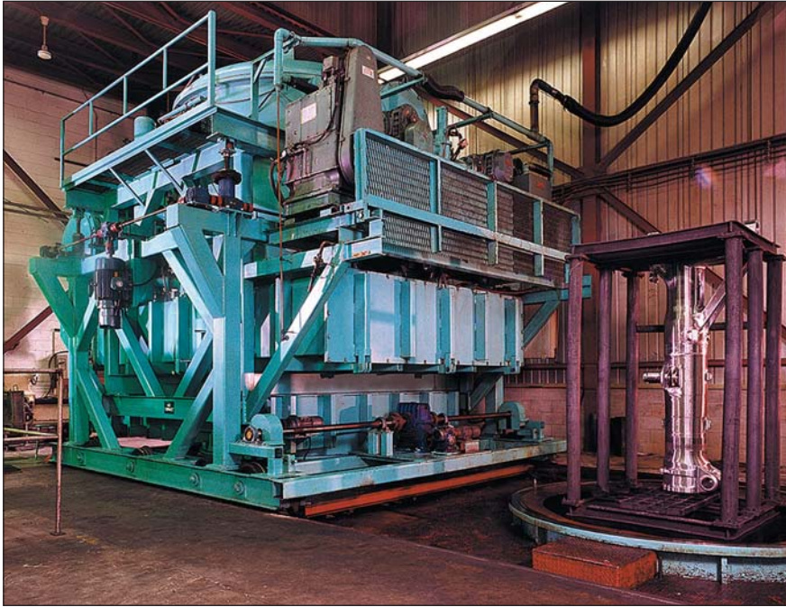
Fig. 2 — Vac Aero Model VAV 72114 MPOGQ vacuum oil quench furnace.
