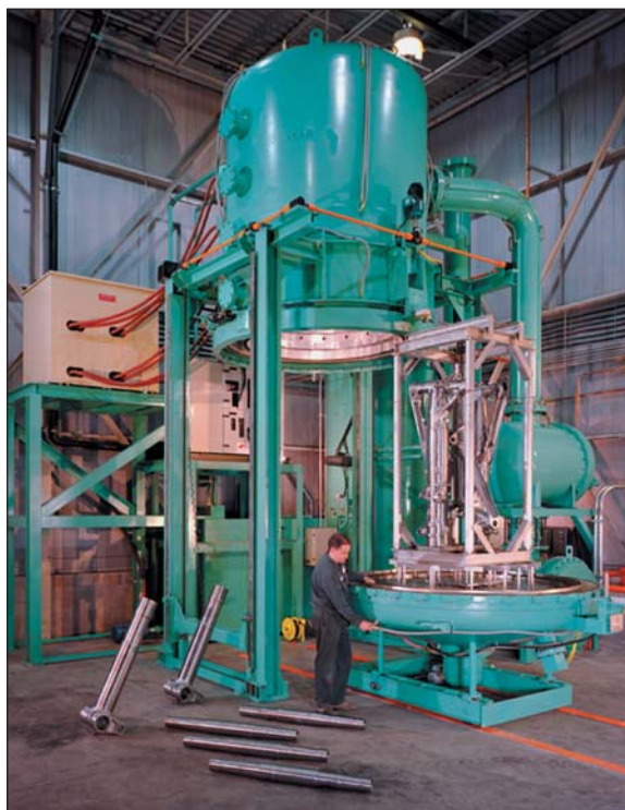
Fig. 4 — Vac Aero Model VAV 72100 MP-10 vacuum gas quench furnace with 10-bar pressure quench capability.
